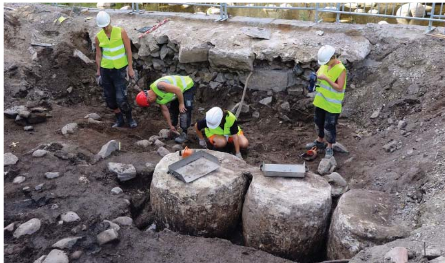
Figure 3a. Photo of the lime barrels (from the left) 4, 3 and 2, which were excavated during the summer of 2014. They have differing sizes but seem to hold similar lime putties. Photo: Kristin Balksten.
