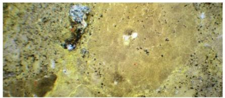
Figure 6.Thin section of unbeaten lime from barrel 1, enlarged 50x in polarization microscope. The lime paste is rather homogeneous and the lime lumps are of the same kind as the rest of the binder showing a rather pure lime. Photo: Kristin Balksten.
